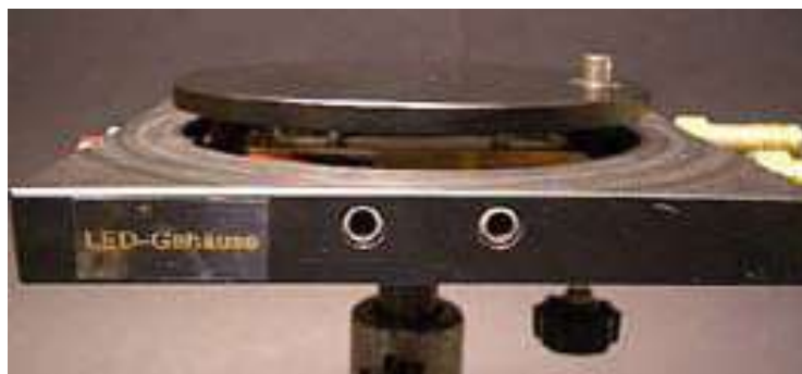
Fig. 6 Connections for plug-in LED illumination
