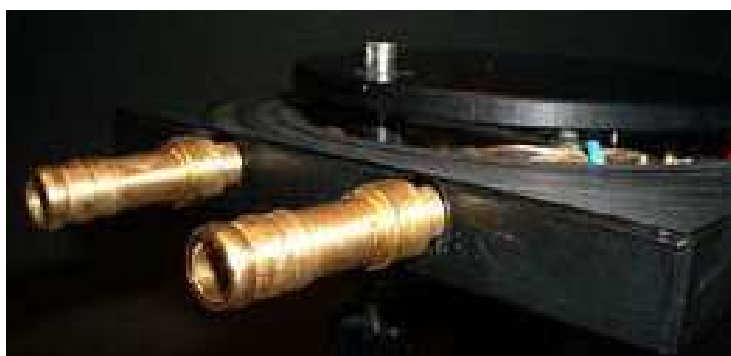
Fig. 7 Connection for cooling water circuit
