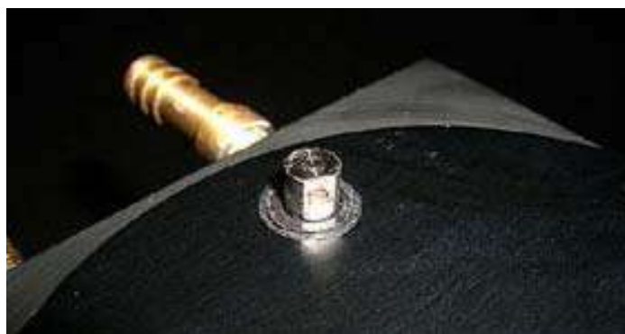
Fig. 3 Insertion of radiation rod in the fog chamber
