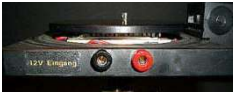
Fig. 5 Connections for supply voltage (12-15V / 8A)
