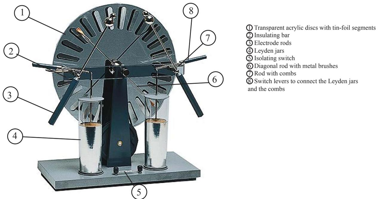
The Wimshurst machine serves as a source of safe, high DC potentials for numerous experiments in the area of electrostatics.
