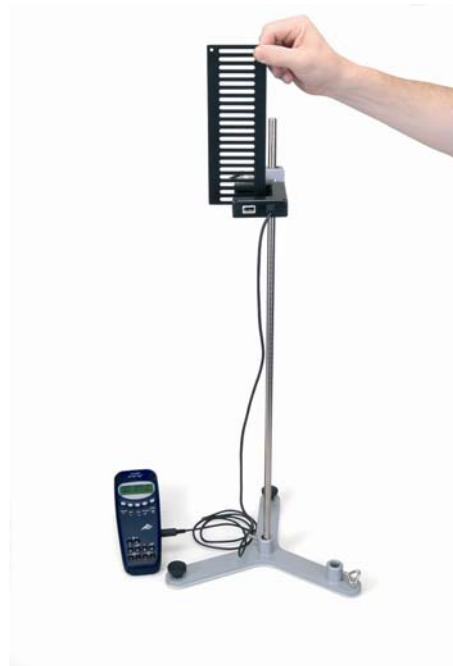
Fig. 1: Measuring free fall
