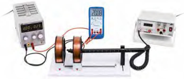
Measurement of Magnetic Field for a Pair of Coils with Variable Separation
