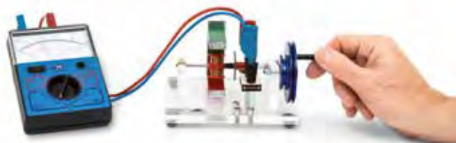
Operating as a DC generator
