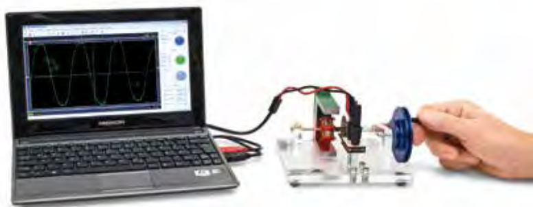
Operating as an AC generator
