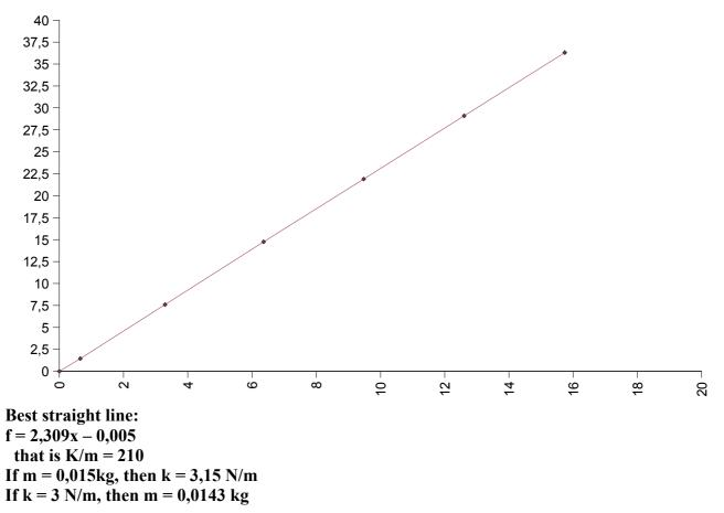
If the theoretical frequencies are precalculated, then k and m must be accurately known.
