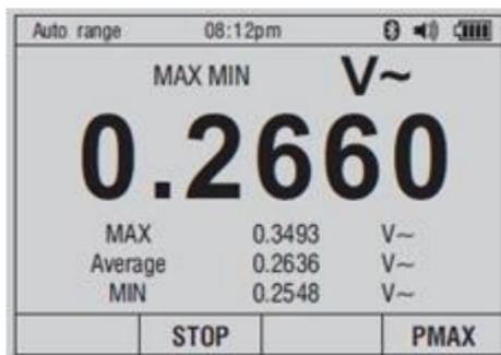
To activate the MAX/MIN mode, press the push-button “F4” (MAX/MIN), at measurement mode.
