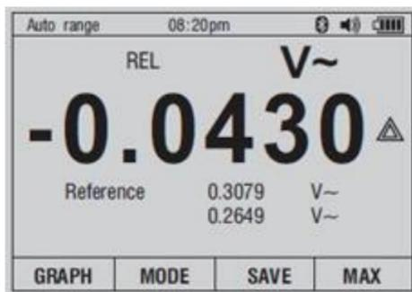
Press the “REL” key, you can measure the relative value and “REL” sign will appear on the LCD display in the relative mode. What is meant by the relative value? Press the “REL” key, the meter make the first measured value into a reference value (You must be decide a reference value as the input signal.), and the meter store the displayed reading as a reference value.
