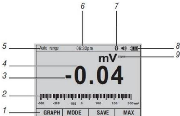
1. Soft key labels Indicates the function of the button just below the displayed label.
