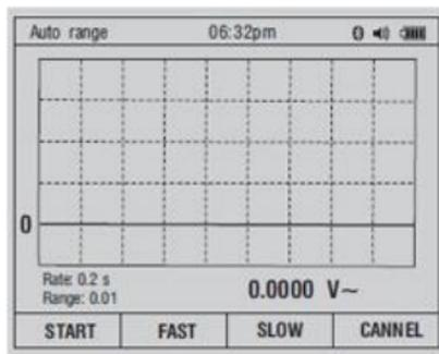
Press soft key "F1" (START) button. Press "F2" (FAST) or "F3" (SLOW) push buttons to select sampling rate. Press "F4" (CANCEL) push button to exit the graphical measurement and return to normal measurement mode.
