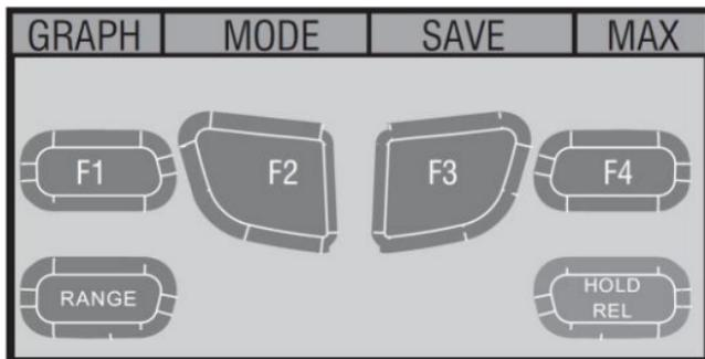
The 6 push buttons on the front of the Meter activate features that augment the function selected using the rotary switch, navigate menus or control power to Meter circuits.
